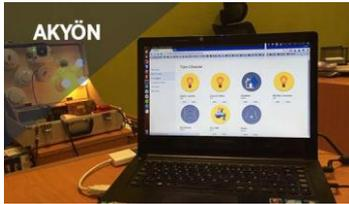
**AKYON- Smart Home Automation System:** Home automation over internet using computer, tablet or mobile phone. User can control remote electric devices (such as lights, oven, heater, A.C.), monitor the condition of home devices and sensor. Users and related persons can be warned in case of emergency.
